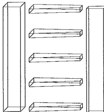
2. Cut out the wedges for the ends and ribs. These will be as wide as the 2x4 at one end and as wide as the 1x4 at the other. The easiest way to cut these, I found, is to cut a 9" plank out of your heavy wood. Then set your table saw's sliding miter gauge at about 2° and cut in alternating directions using your rip fence as a stop. Cut several extras.
