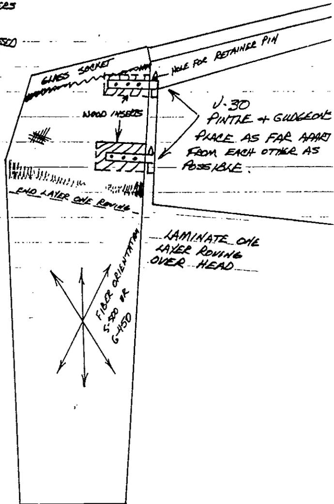
NOTE: RUDDER CAN BE OFFSET TO AVOID BACKSTAY, VANE, ETC, FAVOR THE PORT SIDE FOR THE HAWAII RACE.
