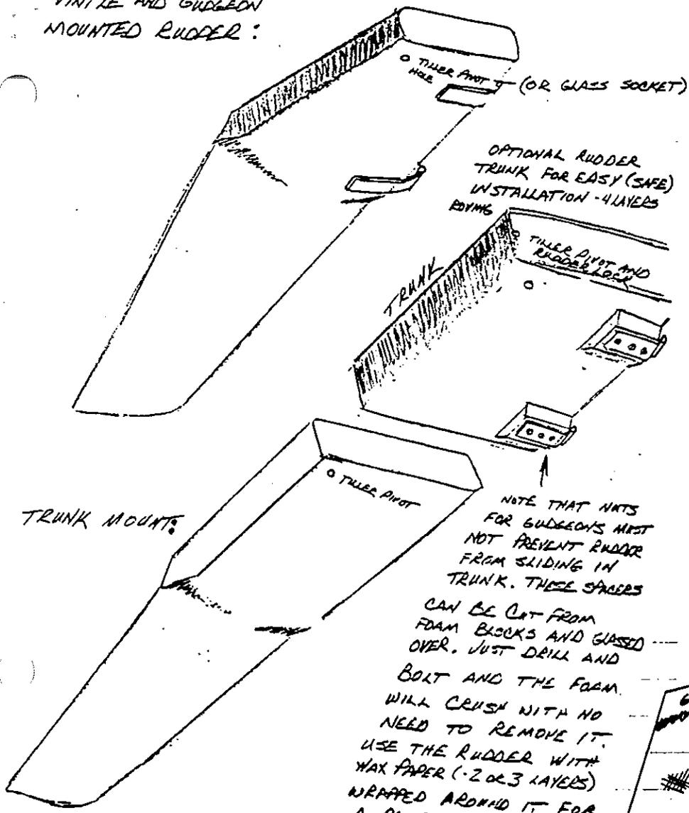
NOTE THAT HNTS FOR GUDGEONS MUST NOT PREVENT RUDDER FROM SLIDING IN TRUNK. THESE SPACERS CAN BE CUT FROM FOAM BLOCKS AND GLASSED OVER. JUST DRILL AND BOLT AND THE FOAM WILL CRUSH WITH NO NEED TO REMOVE IT. USE THE RUDDER WITH WAX PAPER (-2 OR 3 LAYERS) WRAPPED AROUND IT FOR A PLUG.
